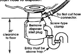
If local plumbing codes permit, dishwasher drain hose may be connected directly to disposer. Most disposers have 7/8" connectors or special connectors are available at plumbing supply houses. Be sure to remove the disposer plug before connecting the drain hose.
